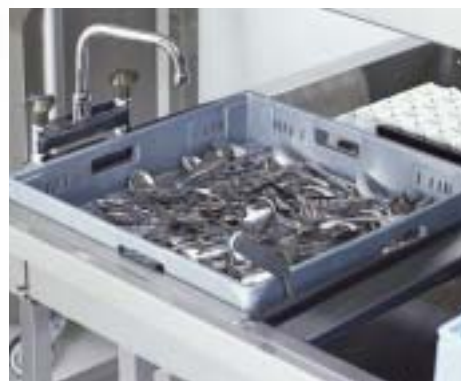
Soaking basin for cutlery is an option that improves washing result of cutlery. Soaking helps to remove the dirt especially if there is a longer accumulating time before washing. Thanks to the lifting handle there is no need to put a hand in the dirty water, but the basket can be smoothly lifted out of the water. Also a faucet with a mixer is available for cutlery soaking basin.
