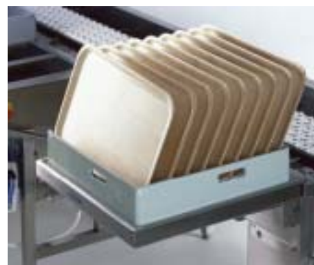
With the help of a tray loading table it is possible to make by-pass of e.g. pre-washing unit with trays. Tray loading table can be folded down when not in use.
