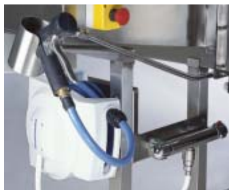
Washing pistol with hose reel is a handy option for cleaning the unit. The hose can be reeled inside the housing when it is not in use. The length of the hose is 8 metres. Thermostatic mixer in the picture is an option. Also regular mixer is available.
