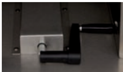
Retractable crank handle (lift 50 mm) for tipping mechanism built into substructure.
