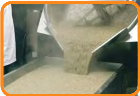
High tilting kettle is fast and easy to empty. Most trolleys fit under kettle's pouring lip.
