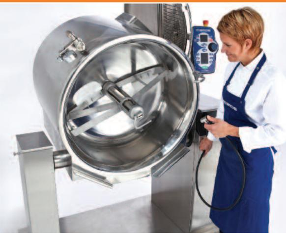
■ Metos ‘combi’ cooking kettles cook, mix and can cool almost any kind of food, providing a huge range of menu options. They ensure optimal energy usage because the energy consumed is directed **ONLY** into the food being cooked *inside* the kettle.
