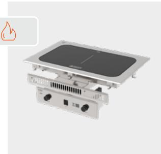
The K|POT® built-in variants, in ceramic heat-retaining, ceramic or induction hob, field dimensions: approx. 607x394x57mm. Suitable for cut-outs: Cover approx. 582x378mm, control approx. 388x152x100mm, front panel approx. 322x85mm. In use with thermoplastes® C with rounded corners & matching GN cooking/buffet lid. Available in 1/1 Gastronorm size in stainless steel. Rated voltage 1N AC 230V 50Hz.
