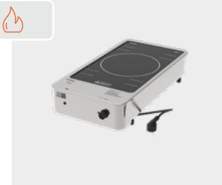
Module with electronically controllable induction ceramic hob (full-surface / round: Ø230mm surface / 2x square: 220x180mm each), controllable with selectable levels 0-9, recessed for safe operation. With ventilated high-performance induction generator. Exact insertion into AST/EST or GN-port, in use with thermoplates® cooking pots. Splash-proof IPX4. Rated voltage 1N AC 230V 50/60Hz.
