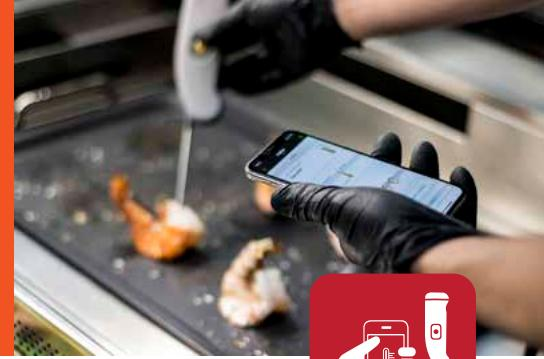
Core temperature sensor - can be retrofitted at any time - order no. 94 01 01 05
