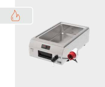
Pasta fryer module, seamlessly welded GN basin 1/1, 200mm with SWISS-PLY multilayer base, powerful heating field underneath. Ventilated, safety drain cock, integrated temperature sensor adjustable +/-1°C. In use with GN hook-in sets in each case. For direct placement in acs front cooking/as table-top unit on worktop. Splash-proof to IPX4. Rated voltage 3N AC 400 V 50/60 Hz.
