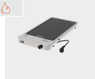
Module for keeping warm at the exact temperature, with infinitely variable & energy-saving ceramic hob (0-800W) with 9 programme levels, recessed for safe operation. Stainless steel housing, with transport-safe, retractable rotary switch. Exact insertion in AST / EST or in GN-port, usually with thermoplates® cooking pots. Splash-proof IPX4. Rated voltage 1N AC 230V 50/60Hz.
