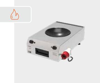
Module with round Ceran cuvette Ø300mm, for safe insertion of a round wok pan, for stepless wok with 11 power levels. With ventilated microprocessor-controlled high-performance induction generator. For precise direct setting in acs-Frontcooking / as table-top unit on worktop. Splash-proof to IPX4.
