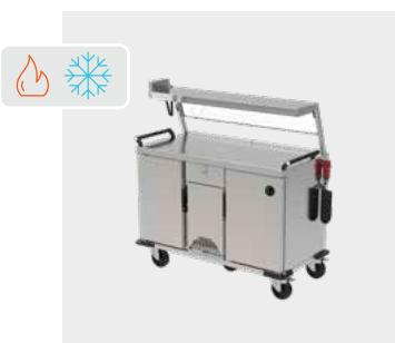
Various compartment combinations for keeping warm/cool & regenerating, bottom 2 compartments each max. 7x GN 1/1 65mm. Type 3 & 5 neutral drawer in the centre. Heat/light bridge, sneeze guard & 3-sided gallery, removable side controls. Cool: +2°C to +14°C. Regenerating: up to +170°C. Rated voltage 1N AC 230V 50Hz / 3N AC 400V 50Hz.
