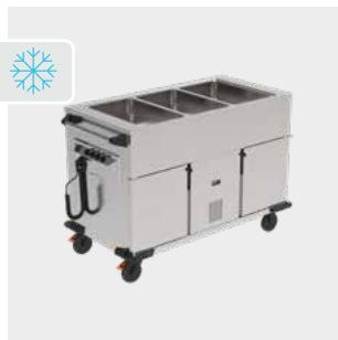
Top 3 deep-drawn GN 1/1 warming trays wet & dry heatable. Bottom 1xheated & 1xcooled GN 1/1 cabinet compartment in H3 (IPX5). Hot: +30°C to 90°C, cold: +2°C to +10°C, 8 deep-drawn bead pairs each. Doors double-walled insulated, self-closing, transport lock. Safety push handle at front, 2 fixed & 2 swivel castors with double stops. Rated voltage 1N AC 230V 50/60Hz.
