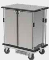
Evaporator in the centre, refrigerator below incl. defrost water evaporator, double-walled EN cabinet compartments & doors. 2-point locking, max. opening angle 270°. 2 full-length round tube push handles on each end. For inserting (lengthwise) EN trays, deep-drawn tray support beading & securing. For transport outside the house, lorry, electric tractor by means of coupling drawbar system.
