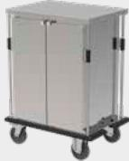
Double-walled insulated EN cabinet compartments & doors, centrally 2 eccentric GN cooling plates & defrost water drain. 2-point locking, max. opening angle 270°. 2 full-length round-tube push handles at each end. Sliding in (lengthwise) of EN trays, deep-drawn tray support ledges & safety catches. For transport outside the house, lorry, electric tractor by means of coupling drawbar system.
