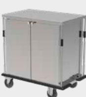
Double-walled insulated EN/GN cabinet compartments & doors, centrally 2 eccentric GN cooling plates & defrost water drain. 2-point locking, max. opening angle 270°. 2 full-length round-tube push handles on each end. Crosswise insertion of EN/GN trays, deep-drawn tray support ledges & safety catches. For transport outside the house, lorry, electric tractor by means of coupling drawbar system.
