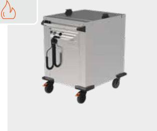
Only for stainless steel baskets (with dimension max. 500x500mm), with stainless steel lid 35mm can be hooked in at the front, stacking height approx. 600mm. Double-walled insulated. With support frame, platform guided tilt- & tilt-proof, max. load 200 kg. Spring force flexibly adjustable, with safety push handle, 4 bumper corners, stainless steel castors (2 swivel & 2 swivel stop castors). Rated voltage 1N AC 230 V 50 Hz.
