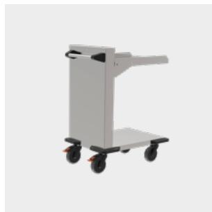
Suitable for baskets (with dimension 500x500mm), stacking height approx. 575mm. Platform guided tilt- & tilt-proof, max. load 200 kg. Spring force flexibly adjustable, with safety push handle, 4 bumper corners, stainless steel castors (2 swivel & 2 swivel stop castors).
