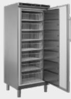
Outer casing galvanised sheet steel, impact/shock resistant powder-coated in white /made of stainless steel. Seamless inner chamber, white plastic with 7 evaporator plates & grid baskets. Lockable door, all-round magnetic chamber seal. Door hinge left/right. Climate class SN-ST.
