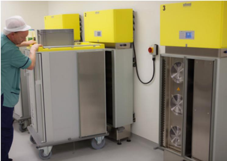
The DSPRO Docking Station is installed in a fixed position to run heating or cooling cycles as required.
