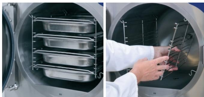
You can simultaneously make different dishes, cook 4x GN 1/1 65 mm or 3x GN 1/1 100mm pans at time.
