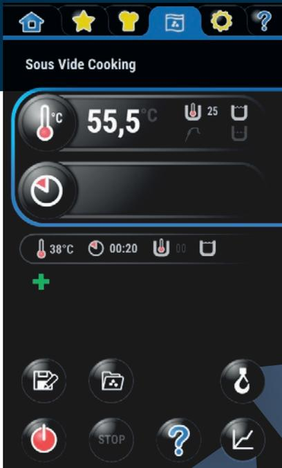
The control panel has a tab for sous vide cooking settings. You can save your own multi-phase programs including cooking and chilling phases.
