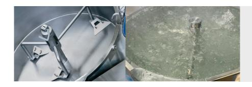
Direct heating while mixing allows rapid boiling of all liquids
