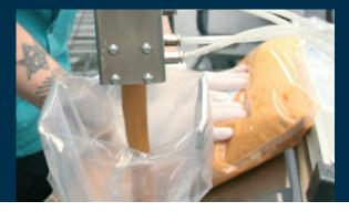
Hot Fill Dos-2 ensures quick and precise dispensing of liquid food products. Soups, sauces and mashed potatoes are filled into bags and containers effortlessly. The built-in scale ensures that weighing of the product happens in one and the same workflow saving time in the kitchen.
