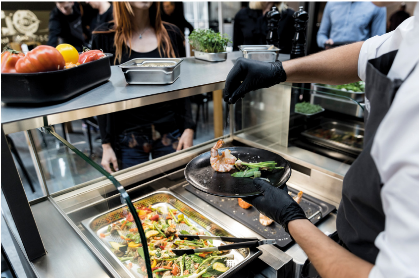
The Rieber Varithek ACS front cooking station offers induction hobs up to 5kW, an induction wok, single or double griddles for steaks, fish or BBQ, Teppanyaki options, plus fryer and pasta cooker configurations.
