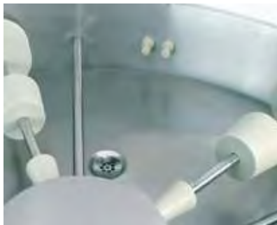
Drain in the bottom of the basin.
