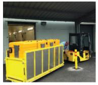
**TROLLEY DOLLY** Pulled by electric vehicle, a specially constructed 'dolly' transports four double Thermoports holding chilled food from a CPU.
