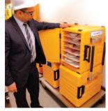
**TRIPLE DECKER FOR PLATED CHILLED MEAL DELIVERY** Three and two-tier Thermoport trolleys used to transport trayed chilled meals and foods. Trolleys are configured to suit different numbers at the service points, in this case, internally, but heavier duty castors can be used to cope with outside paths and roadways.
