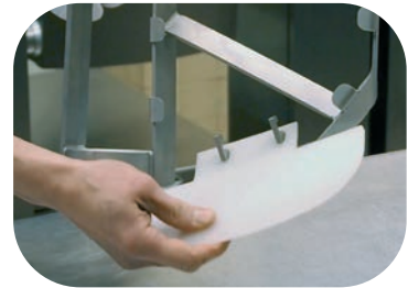
Easily removable scrapers. All parts are machine washable.
