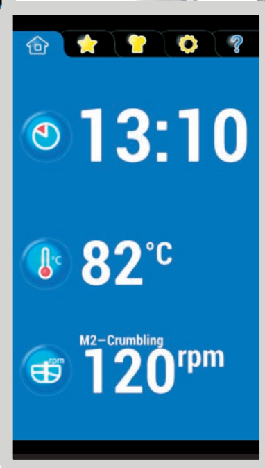
Various phases are displayed on the status display. Audible signals inform the user about any required actions.
