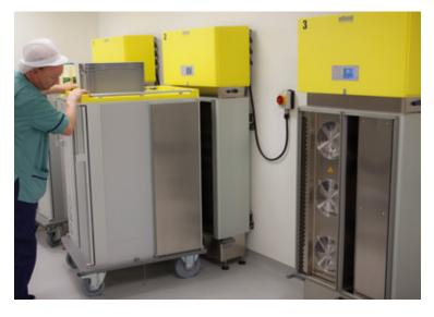
The DSPRO Docking Station is installed in a fixed position to run heating or cooling cycles as required.
